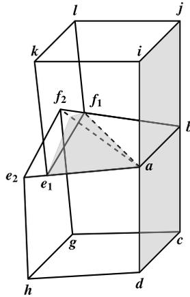
**Fig. 12.** Overlapping region formed between neighboring flux volumes  $abcde_2f_2gh$  and  $baijf_1e_1kl$  when simple rescaling (i.e., time-step adjustment) is used to create conservative fluxes. The face with vertices  $abf_1e_1$  is triangulated with diagonal  $af_1$ . Rescaling the bottom flux volume moves the projected vertices creating the shaded overlapping region.
