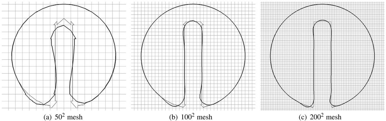
Fig. 16. Zalesak's disk after one rotation of various meshes. The thick line is the computed solution and the thin line indicates the initial condition on each mesh.
