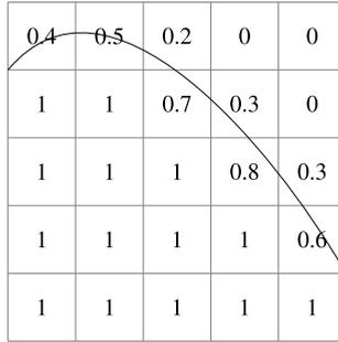
Fig. 4. Representation of interface (solid line) using a VOF scheme. Liquid volume fraction  $\alpha$  shown with numbers.
