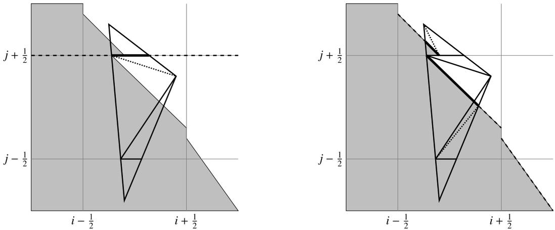
(c) Simplices in (b) are cut by plane at  $j + \frac{1}{2}$  (thick solid line). Resulting shapes are partitioned into simplices (dotted line) that are unique to one computational cell.
