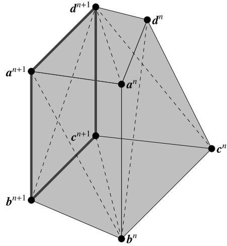
(b) Discrete representation of a flux volume using six simplices.
