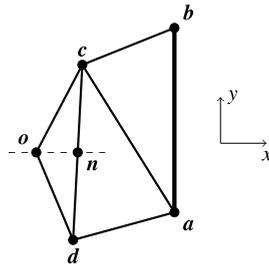
**Fig. 13.** Modification of two-dimensional flux volume to create solenoidal flux. Original flux volume associated with face  $ab$  has vertices  $abcd$ . The additional simplex with vertices  $cdo$  is added.
