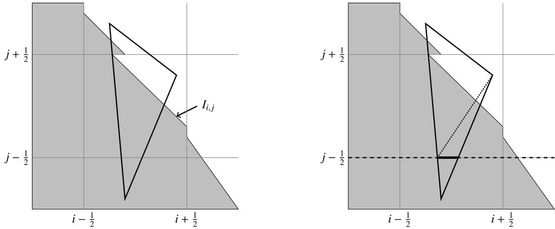
(a) Original simplex and PLIC reconstruction of interface indicated with  $I_{i,j}$  in cell  $i, j$ .
