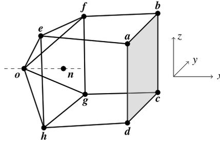
**Fig. 14.** Modification of three-dimensional flux volume to create solenoidal flux. Original flux volume associated with face *abcd* has vertices *abcdefgh*. Two additional simplices with vertices *efho* and *fgho* are added if six simplices are used to discretize the original volume.
