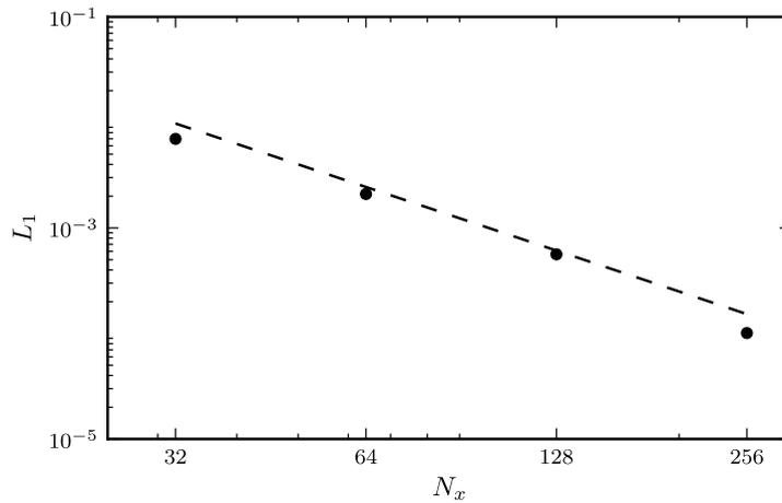
Fig. 21. Convergence of the  $E_{\text{shape}}$  error for the three-dimensional deformation simulations. The dashed line shows second-order convergence.
