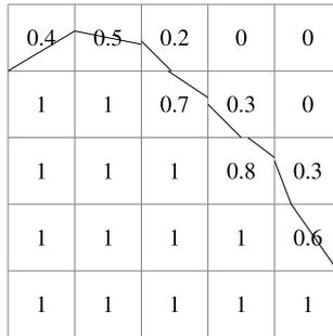
Fig. 5. Example of PLIC reconstruction of interface from liquid volume fraction.
