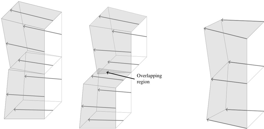
**Fig. 1.** Example of methods used to compute geometric fluxes. Velocity vectors used to construct fluxes are shown with arrows. Fluxes are shaded.
