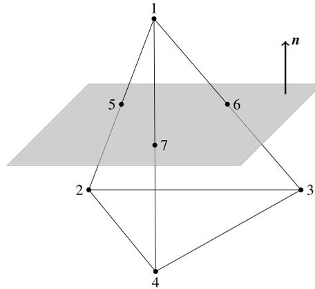
Fig. 15. Example simplex and cut-plane classified as Case = 2. Vertices indicated with their index number.
