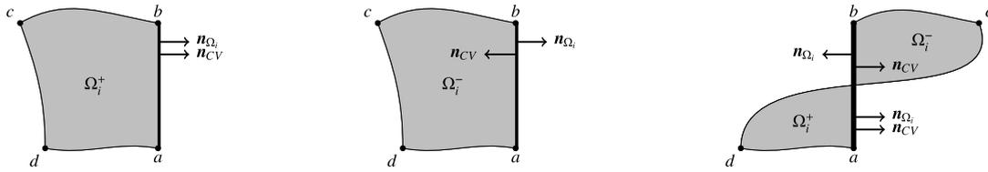
(a) Simple example with positive flux volume,  $\Omega_i^- = \emptyset$ . (b) Simple example with negative flux volume,  $\Omega_i^+ = \emptyset$ . (c) Example with crossed flux volume with both positive and negative regions.
