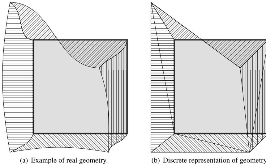
**Fig. 6.** Example geometry of the two-dimensional flux volume associated with a computational cell (shaded). (a) Shows an example of a realistic geometry where the four flux volumes (indicated with lines) do not have straight edges. (b) Shows how the real geometry can be approximated using two simplices per flux volume.
