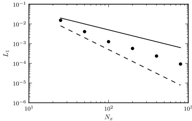
**Fig. 17.** Convergence of the  $E_{\text{shape}}$  error at the end of the simulation for the transport of Zalesak’s disk. Solid and dashed lines show first- and second-order convergence, respectively.
