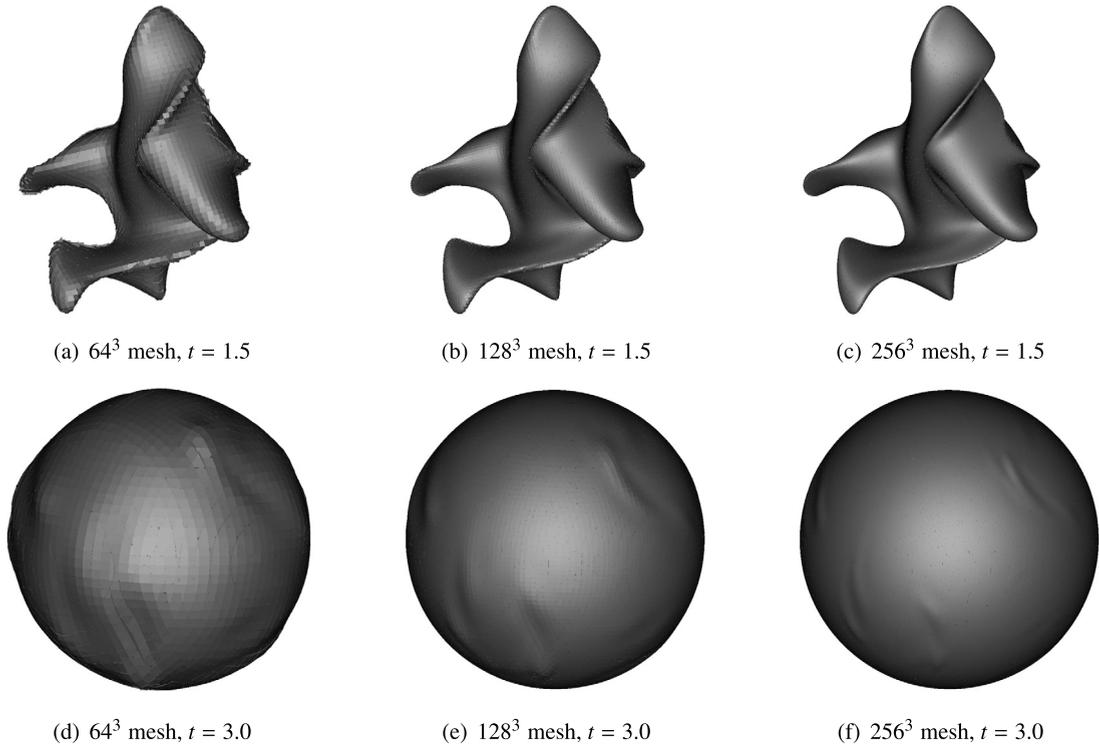
**Fig. 22.** Gas-liquid interface for the droplet in homogeneous isotropic turbulence test on various meshes. Snapshots on the top show the droplet at maximum deformation ( $t = 1.5$ ). The droplets at the end of the simulation ( $t = 3$ ) are shown on the bottom.
