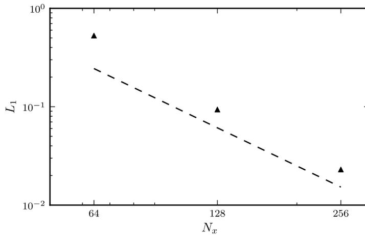
**Fig. 23.** Convergence of the  $E_{\text{shape}}$  error for the simulation of the droplet in homogeneous isotropic turbulence. Dashed line shows second-order convergence.
