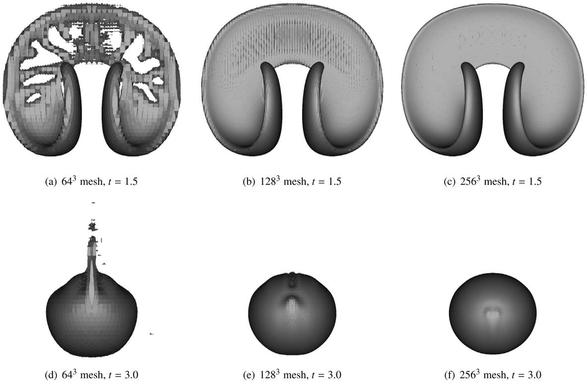
Fig. 20. PLIC interface for the droplet in three-dimensional deformation flow on various meshes. Snapshots on the top show the droplet at maximum deformation ( $t = 1.5$ ). The droplets at the end of the simulation ( $t = 3$ ) are shown on the bottom.
