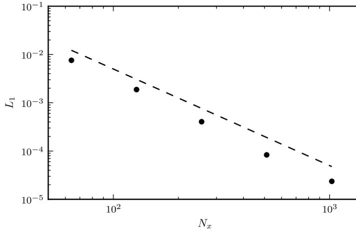
Fig. 19. Convergence of the  $E_{\text{shape}}$  error at the end of the two-dimensional deformation test. Dashed line shows second-order convergence.
