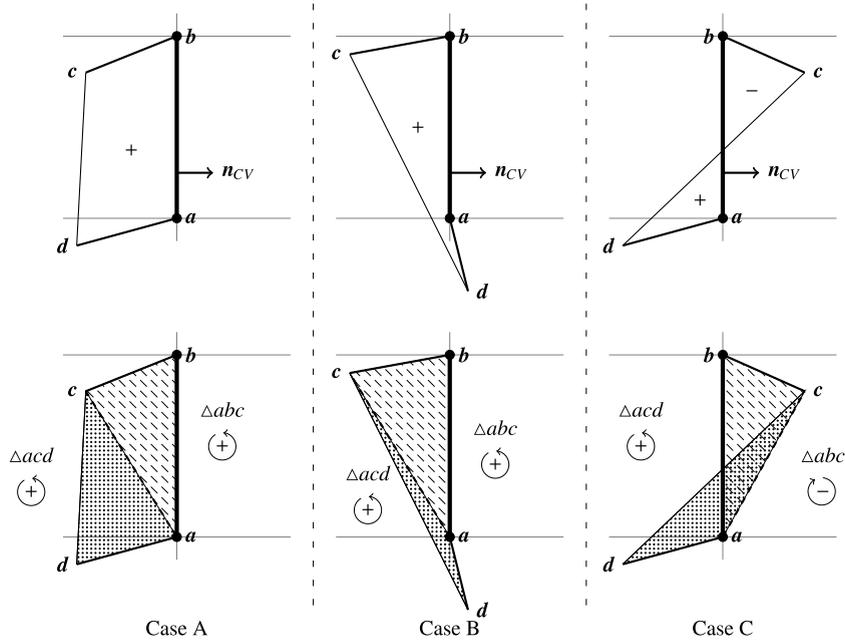
Fig. 8. Example of the discrete representation of two-dimensional flux volumes using signed simplices.
