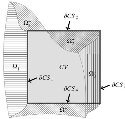
**Fig. 2.** Example geometry used to construct the flux volumes. The control volume  $CV$  is shown as the shaded region. The bounding surface of  $CV$  has been partitioned into four sub-surfaces  $\partial CS_i$  with  $i = 1, \dots, 4$ . Associated with each sub-surface is the flux volume  $\Omega_i$ . Each flux volume is indicated with a different pattern of lines.
