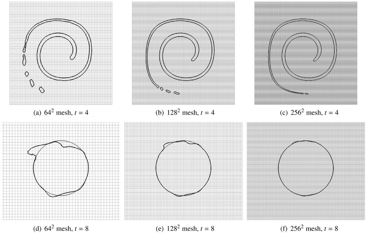
**Fig. 18.** Effect of mesh size on two-dimensional deformation test case. The top images show the disk at maximum deformation. The bottom images show the result at the end of the simulation with the thick line and the thin line indicates the initial condition.
